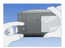
Slide the film door latch; the door will pop open. Lift the door up until it stops. Hold the film pack by its edges with the arrows facing you. Slide the pack into the camera in the direction of the arrows, as shown.
